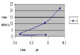
pH progressively increased during bioleaching due to alumina solubility and reached a maximum of 9.47 in case of 0.3g carbon source where alumina % being 15.50 after 15 days of incubation and then decreased. Such an effect can be justified that increasing in pH results in the ability of metabolite to dissolve alumina .Thus after 20days there was no complexation reaction occurred between alumina and organic acids released by the microorganisms.
